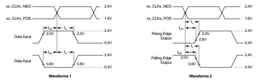
**Figure 5. Timing Measurement Waveforms**
